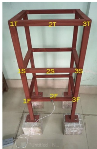
Fig. 3 Test Frame with sensor mounted at 2F
