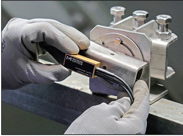
Fig. 3. The installation of the LUNA os7520 fiber-optic accelerometers.
