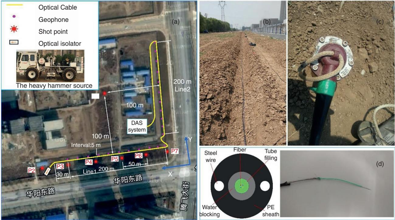
**Figure 4.7** Field trial of near-surface seismic experiment. (a) Plan view of experimental layout, (b) photo of the buried fiber optic cable, (c) photo of a 3C geophone, and (d) structure of the fiber optic cable.
