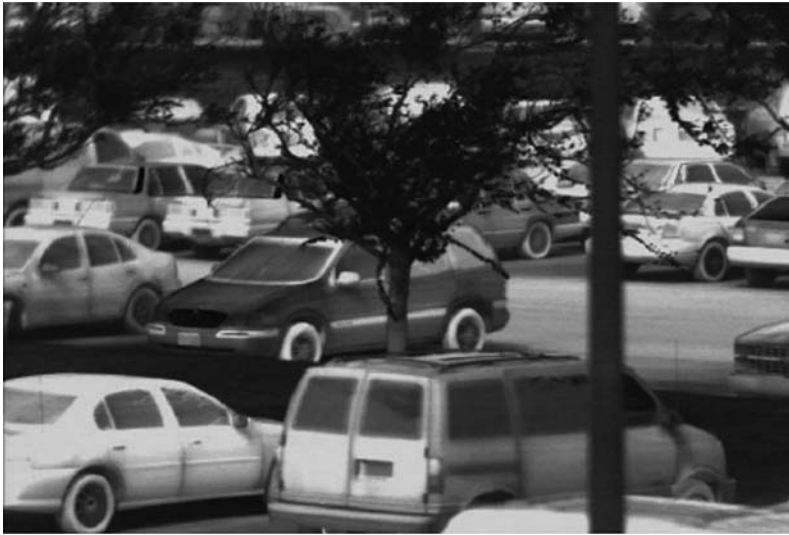
Figure 9.16 IR image taken by a 480 \times 640 pixel microbolometer. These devices can detect temperature variations smaller than 0.1 K. (Reprinted from Ref. 67.)
