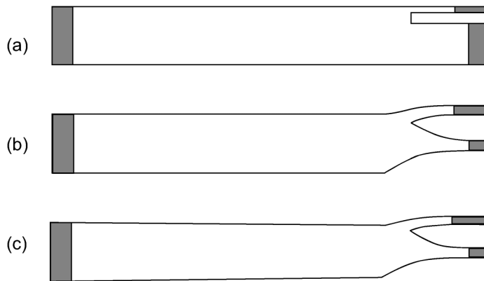
Figure 5.18 Schematic geometry of drift/readout regions of SPRITE detectors: (a) straight/bifurcated, (b) straight/horn, and (c) tapered/horn. (Reprinted from Ref. 7 with permission from Elsevier.)
