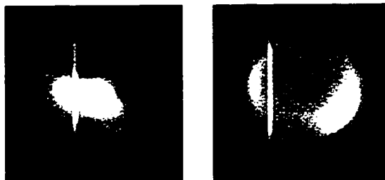
Fig. 7- 1: MBE grown VCSELs after 72-hour, 30 mA burn-in. Note that the features observed at 780 nm (left) could be observed across all wavelengths from 750 - 790 nm. Little contrast is obtainable at 850 nm (right). (The white line is from video system; the dot on upper part of right image is a dust spot.)
