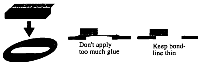
Fig. B- 6: Sample being bonded to TEM grid (left). If excess glue is used (center), a meniscus forms with glue across the center of the sample (which will subsequently prevent the sample from being electron transparent). A thin bond-line is needed (right) to prevent this.
