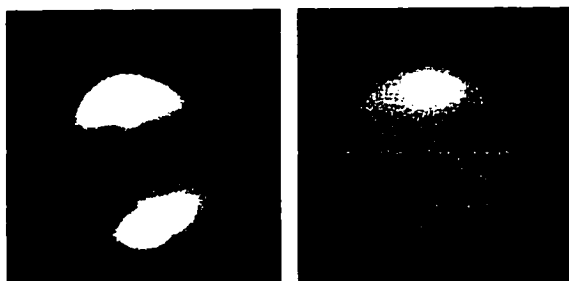
Fig. 7- 3: MBE VCSEL after aging for thousands of hours. 780 nm image (left) shows a dark "band" across the center with two especially dark areas in it. Unfiltered image (right) shows little contrast, as before.
