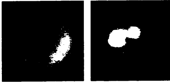
Fig. G - 12: Filtered EL of lasing VCSEL. 850 nm image (right) shows lasing filaments, concentrated at the top of the device. 780 nm image (left) shows dark areas of reduced spontaneous emission where the lasing mode has depleted the carrier population.
