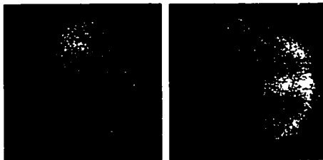
Fig. 7- 7: Dielectric mirror VCSEL after rapid aging. 780 nm image is seen at left; unlike previous devices from this chapter, independent image contrast is seen in the 830 nm image (right), showing what appear to be \langle 110 \rangle DLD networks growing from the left of the device toward the right.
