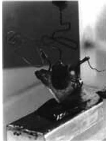
Figure 5.2 The first point-contact transistor, which was invented at Bell Laboratories on 23 December 1947 (reprinted with permission from Alcatel-Lucent).
