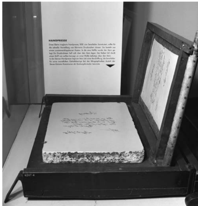
Figure 2.3 Lithographic stone and small hand press constructed by Alois Senefelder in 1818 and used for fast production of lithographic prints. Note the copy made from the handwritten note on the lithographic stone. (Printed with permission from the Deutsches Museum, Munich.)
