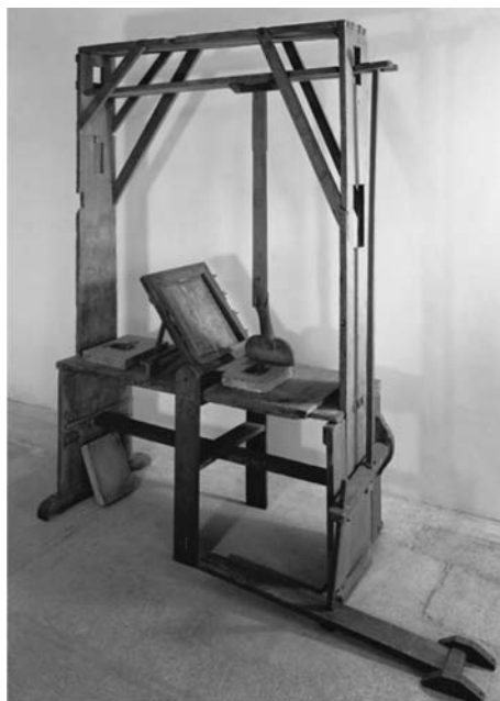
Figure 2.2 Wooden lithographic press constructed by Alois Senefelder and used in his invention of lithography (printed with permission from the Deutsches Museum, Munich).
