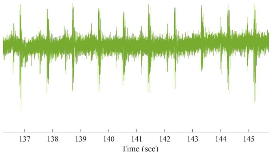
**Figure 2. MatLab view of one set of 10 hammer hits in the sand trench.**
