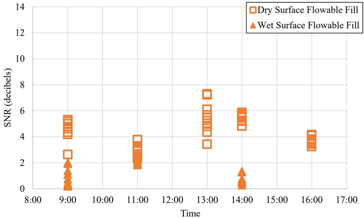
Figure 5. Signal-to-Noise (SNR) Ratio in Flowable Fill Trench.
