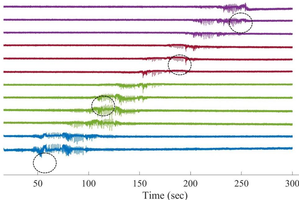
**Figure 1. MATLAB plot showing hammer hits on 11 channels in the testbed. Dark blue for gravel, green for sand, dark red for flowable fill, and purple for the native loess material.**
