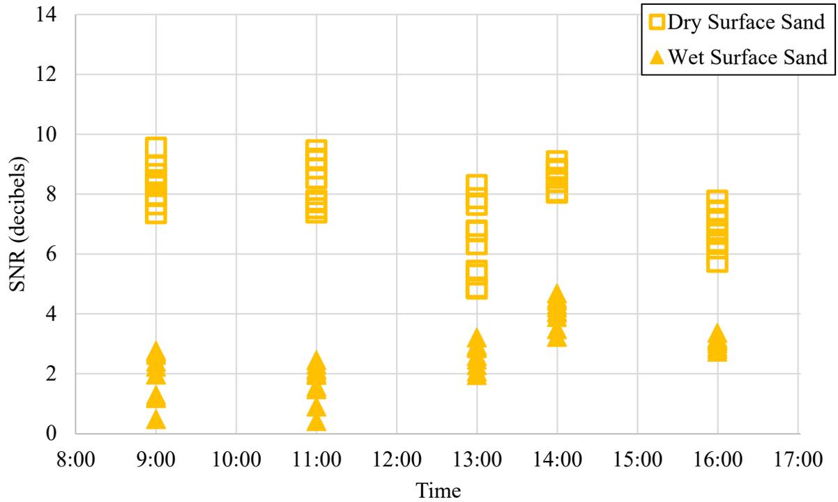
Figure 4. Signal-to-Noise (SNR) Ratio in Sand Trench.
