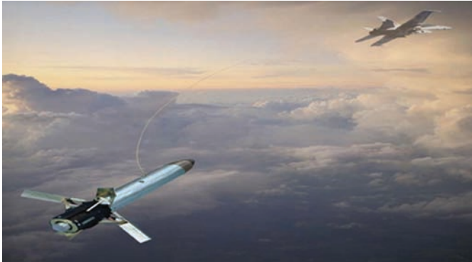
Figure 8.9 BAE Systems' AN/ALE-55 fiber-optic towed decoy (shown on left) is an RF self-protection decoy for aircraft. (Image from Naval Research Lab website: https://www.nrl.navy.mil/tewd/organization/5710/5713 .)
