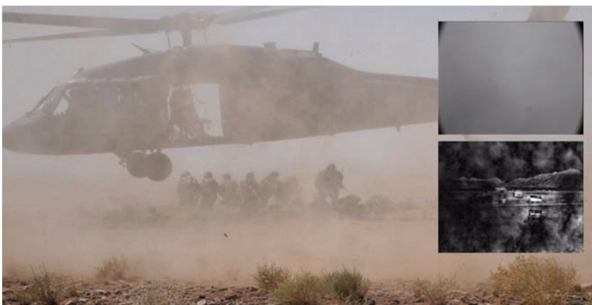
Figure A1.6 NVESD develops advanced camera capabilities and algorithms to increase flight safety in degraded visual environments, such as brownout. Visibility to the pilot is significantly improved in the processed FLIR imagery; see lower right insert. (U.S. Army photo.)
