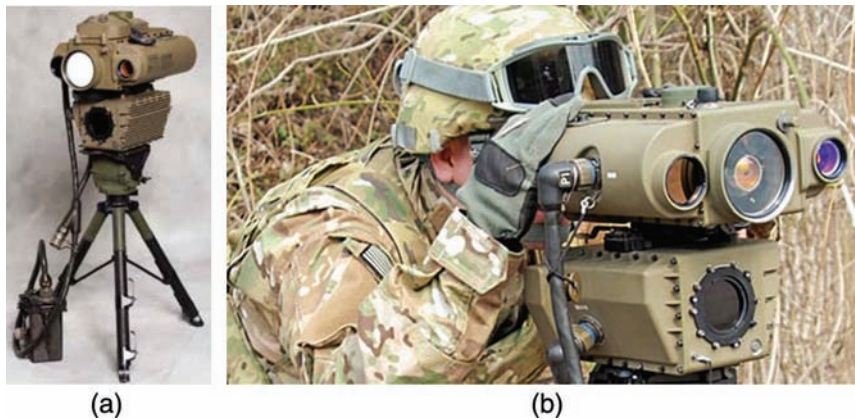
Figure 5.8 (a) Northrop Grumman Lightweight Laser Designator Rangefinder with High Resolution (LLDR-2H) combines multiple sensors into a single package. (b) Northrop Grumman AN/PED-1 LLDR. [Photographs from: http://www.northropgrumman.com/Capabilities/ANPED1LLDR/Pages/default.aspx (accessed Nov. 25, 2017). Used by permission.]
