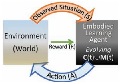
Figure 6.9 Reinforcement learning is learning how to act to maximize a numerical reward. An agent selects an action, the action causes changes to the perceived world (environment) that are then analyzed; a reward is returned to the agent, which then leads to a new action, and so the cycle continues.
