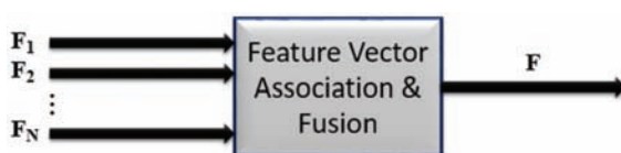
Figure 5.12 Feature fusion combines N feature vectors into a single feature vector F .
