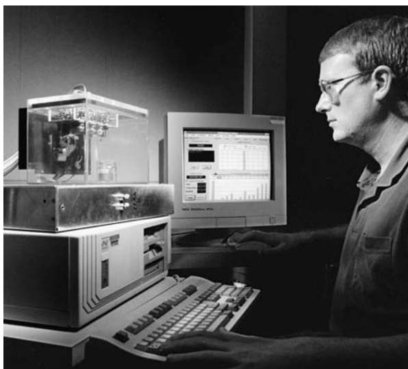
Figure 10.26 Photograph of the prototype electronic nose in operation.
