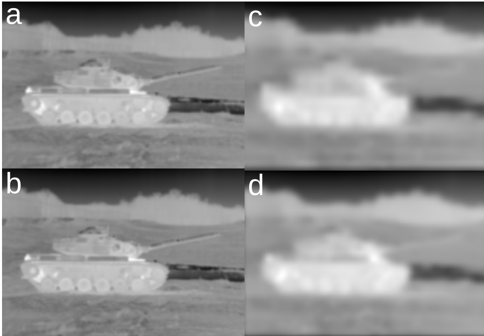
Figure 8.7 In (a) and (b), the target is at 1.1 km. In (c) and (d), the target is at 4.3 km; (c) and (d) are enlarged for comparison. The MTF is the same in all images. However, in (b) and (d), the sampling is better than in (a) and (c). Notice that image quality in (d) is substantially better than in (c). This improvement results solely from better sampling.
