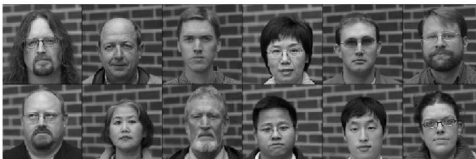
Figure 6.14 Set of 12 faces that look sufficiently diverse to be a good test set. However, with this test set, range performance can only be modeled by using the frequency spectrum of the faces as target contrast. In other words, the target set is not sufficiently diverse that imager resolution alone predicts performance.
