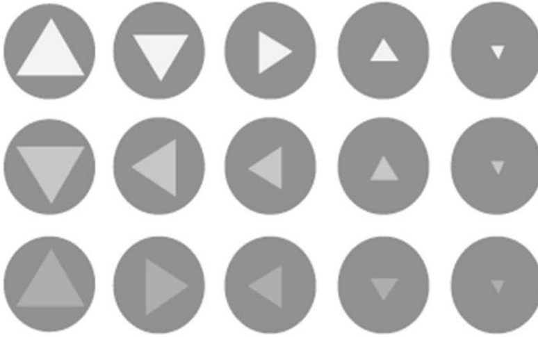
Figure 9.16 Triangle orientation discrimination (TOD) patterns. The operator must call the correct orientation. Using a forced-choice test reduces the errors associated with a subjective judgment such as calling bar visibility.
