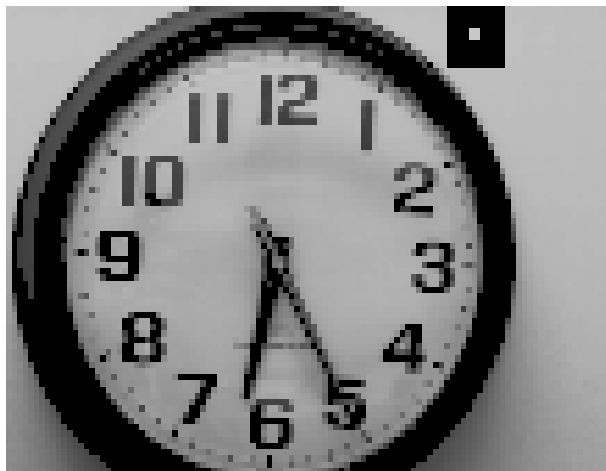
Figure 3.15 Clock image in Fig. 3.1 downsampled by four in each direction; sample frequency is now 0.42 cy/mrad. The display pixel has not changed from Fig. 3.12. Sampling artifacts have appeared. The intensity and thickness of lines varies across the picture, and some of the minute markings are missing completely.
