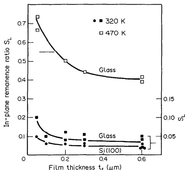
Figure 1. In-plane remanence ratio  $S_L$  vs film thickness  $t_f$  of Co-23at% Cr layers on different substrates.
