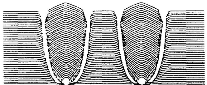
Figure 4. Pair of hillocks calculated in the 'global' shadowing model with incidence angles  $\phi$  for the oncoming atoms in the range of  $60^\circ < |\phi| < 75^\circ$  to the surface normal (lines represent the temporal development of the surface of the film as well as of the nodules).
