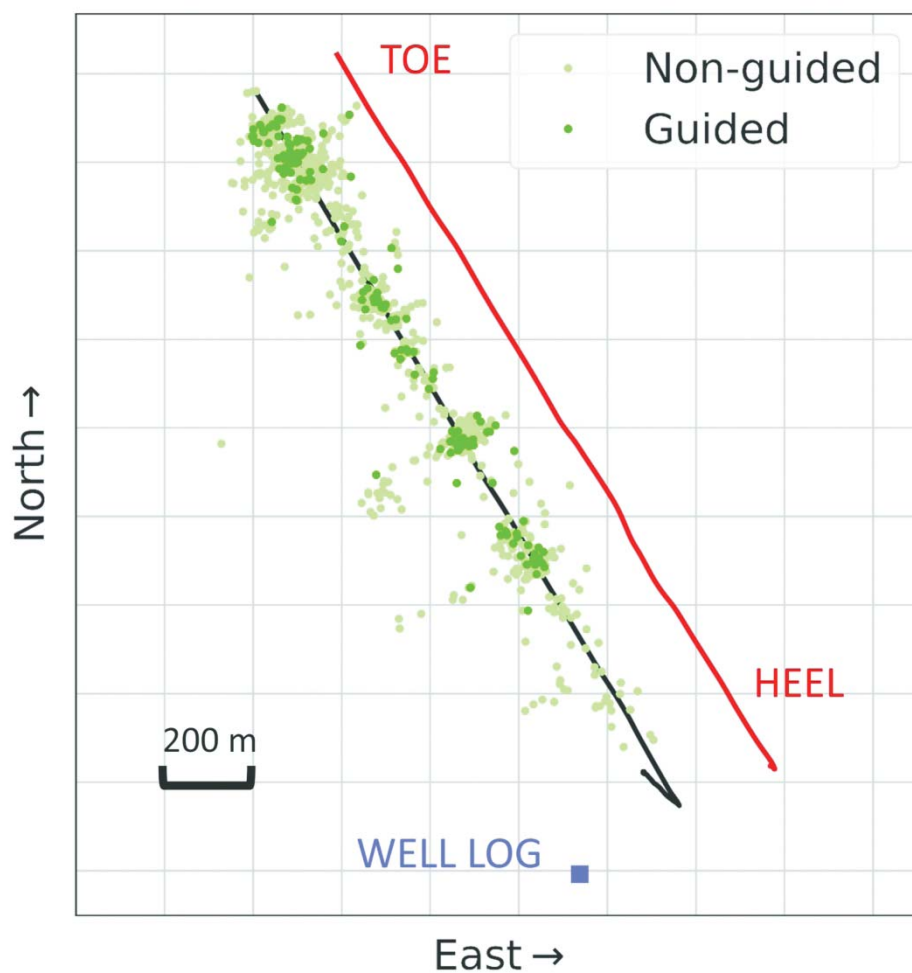
Figure 8. Map view of the microseismic events that occurred during the hydraulic fracturing operations in the Eagle Ford project. Locations were obtained from surface geophone processing. Events are color-coded to indicate whether energetic guided waves are observed (Huff et al., 2020). The horizontal section of the DAS monitor well (red curve), the horizontal section of the treatment well (black curve), and a vertical well (blue square) that was logged are also shown.
