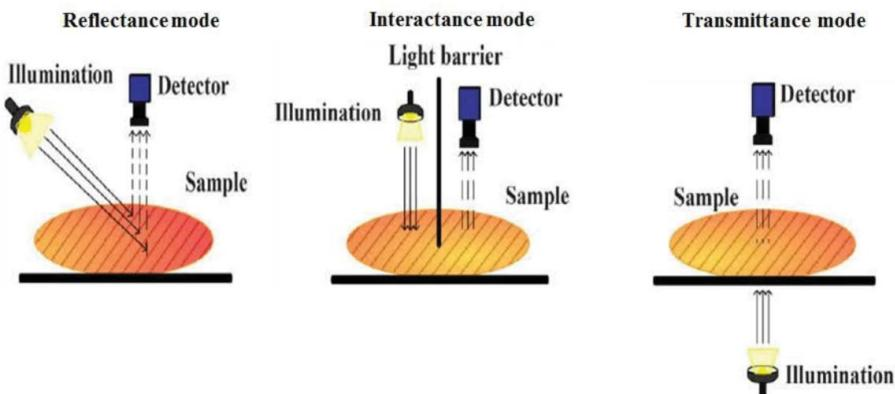
**Figure 3.** Mode of data acquisition in the VIS/IR system (106).
