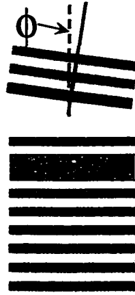
Figure 6.15 Tunable VCSEL structure with a tilted top DBR
