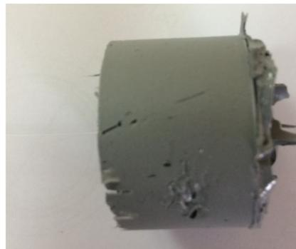
iii) Side view : hole RTV3145 packaged fibre
