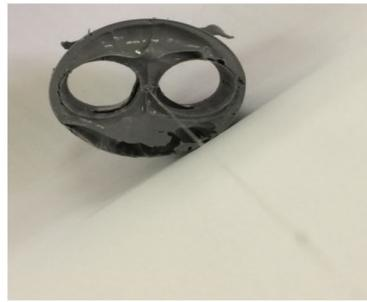
i) Front view: side hole RTV3145 packaged fibre
