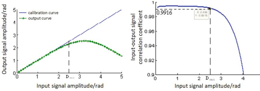
(a) Amplitude Relation Diagram of Output-Input Signal in PGC Demodulation System
