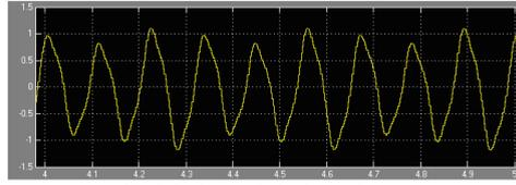
(a) After the whole process of PGC demodulation, the system output signal waveform
