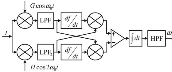
Fig. 1. Principle block diagram of PGC demodulation
