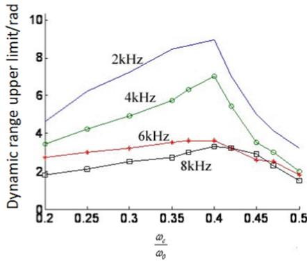
**Fig. 3.** The influence of different cut-off frequencies of filters on the upper limit of dynamic range of the system
