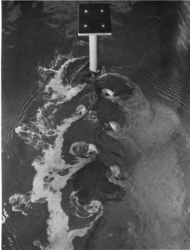
FIG. 9. Surface flow patterns. Self excited oscillations cross-flow.
