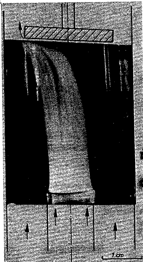
FIG. 12. — Experimental flow pattern, conditions as in Figure 8 but the deposition surface is arranged oblique. \text{TiCl}_4 - \text{H}_2\text{O} in the inner tube.
