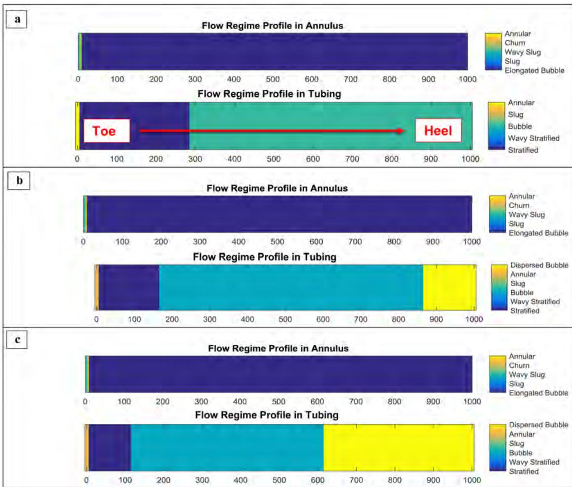
Figure 15—Flow regime along 1000 m well with tubing deployed completion completion, 4 ½ inch diameter tubing and 7 inch screen for steam breakthrough at toe; top figure is for annulus and bottom figure is for tubing; (a) liquid rate=1000 bbl/d, (b) liquid rate=3000 bbl/d, (c) liquid rate=6000 bbl/d
