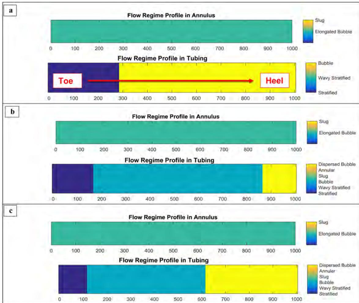
Figure 12—Flow regime along 1000 m well with tubing deployed completion design, 4 ½ inch diameter tubing and 7 inch screen for no steam breakthrough; top figure is for annulus and bottom figure is for tubing; (a) liquid rate=1000 bbl/d, (b) liquid rate=3000 bbl/d, (c) liquid rate=6000 bbl/d
