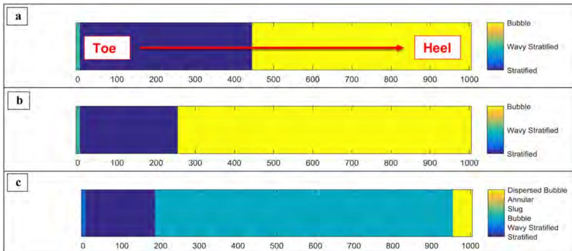
Figure 19—Flow regime along 1000 m well with liner deployed completion design, 7 inch diameter screen with steam breakthrough at toe; (a) liquid rate=1000 bbl/d, (b) liquid rate=3000 bbl/d, (c) liquid rate=6000 bbl/d
