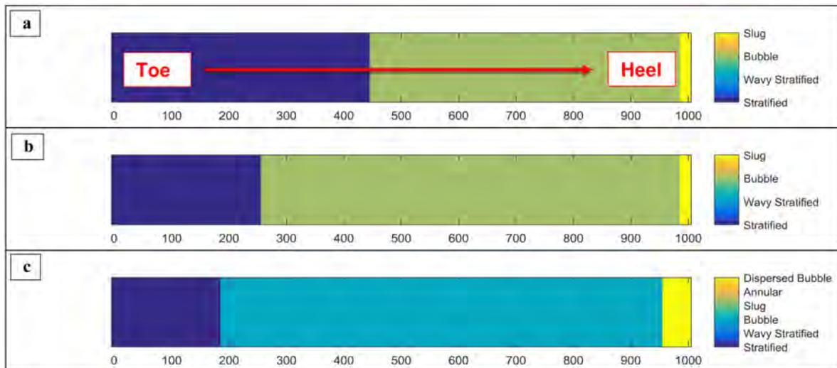
Figure 17—Flow regime along 1000 m well with liner deployed completion design, 7 inch diameter screen with steam breakthrough at heel; (a) liquid rate=1000 bbl/d, (b) liquid rate=3000 bbl/d, (c) liquid rate=6000 bbl/d
