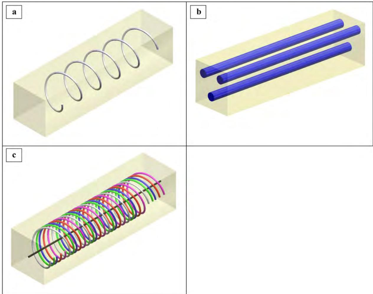
Figure 3—Multicomponent DAS configurations (a) helical optical fibers, (b) multiple parallel optical fibers (c) straight optical fiber inserted into five equally spaced helical fibers
