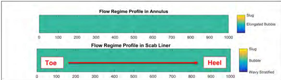
Figure 8—Flow regime along 1000 m well with scab liner design, 4 ½ inch diameter scab liner and 7 inch screen for no steam breakthrough; top figure is for annulus and bottom figure is for scab liner
