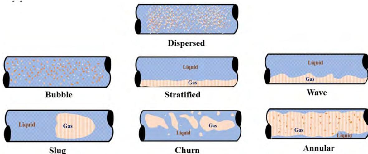
**Figure 5—Possible flow regimes that might be formed inside the pipe and annulus.**
