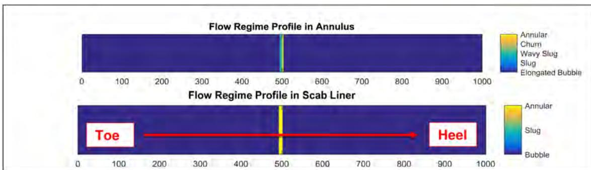
Figure 10—Flow regime along 1000 m well with scab liner design, 4 ½ inch diameter scab liner and 7 inch screen for steam breakthrough in the middle; top figure is for annulus and bottom figure is for scab liner
