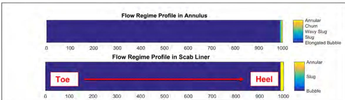
Figure 9—Flow regime along 1000 m well with scab liner design, 4 ½ inch diameter scab liner and 7 inch screen for steam breakthrough at heel; top figure is for annulus and bottom figure is for scab liner
