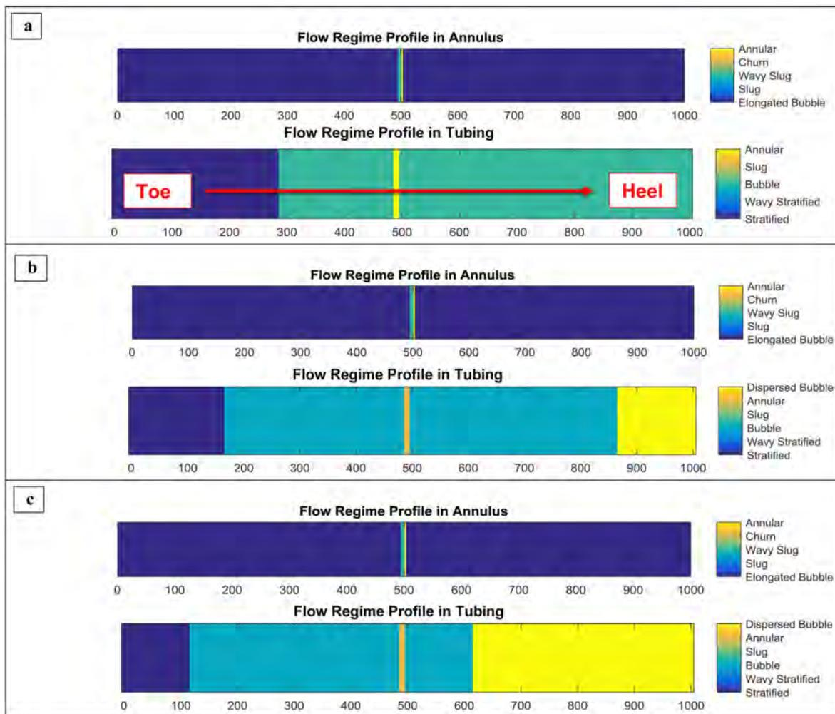
Figure 14—Flow regime along 1000 m well with tubing deployed completion completion, 4 ½ inch diameter tubing and 7 inch screen for steam breakthrough in the middle; top figure is for annulus and bottom figure is for tubing; (a) liquid rate=1000 bbl/d, (b) liquid rate=3000 bbl/d, (c) liquid rate=6000 bbl/d
