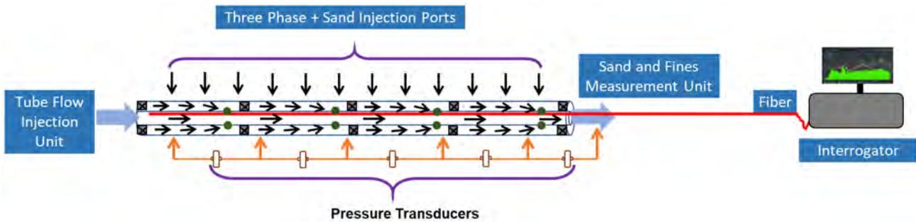
Figure 22—Design 3: tubing deployed completion
