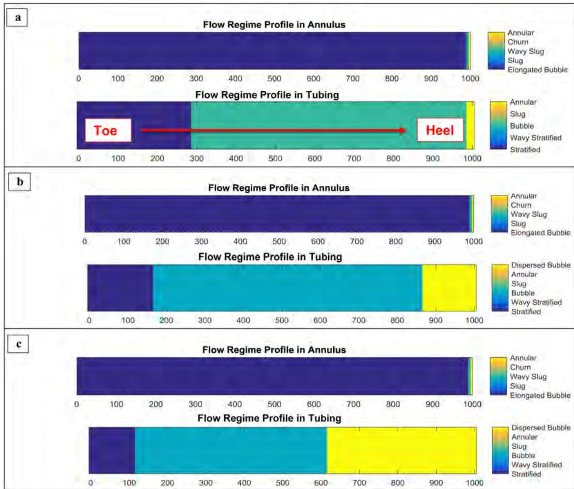
Figure 13—Flow regime along 1000 m well with tubing deployed completion design, 4 ½ inch diameter tubing and 7 inch screen for steam breakthrough at heel; top figure is for annulus and bottom figure is for tubing; (a) liquid rate=1000 bbl/d, (b) liquid rate=3000 bbl/d, (c) liquid rate=6000 bbl/d
