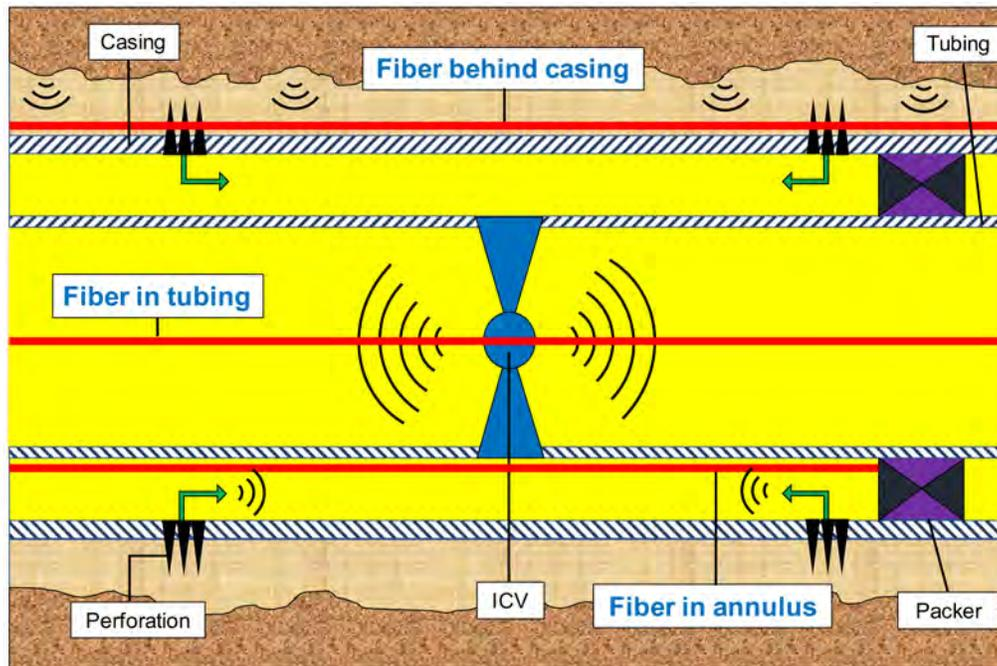
Figure 2—Fiber optics installation in the wellbore (Soroush et al. (2019))
