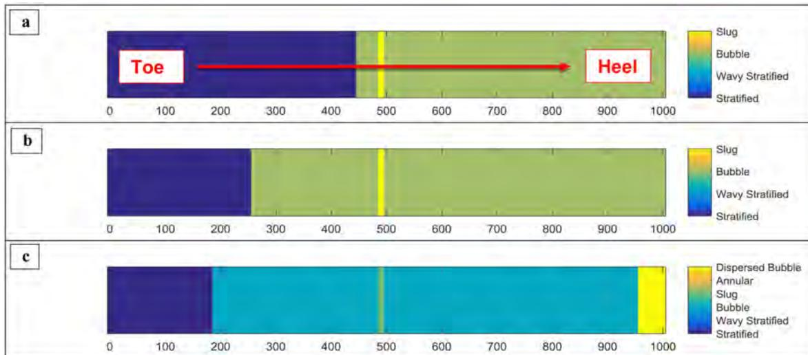
Figure 18—Flow regime along 1000 m well with liner deployed completion design, 7 inch diameter screen with steam breakthrough in the middle; (a) liquid rate=1000 bbl/d, (b) liquid rate=3000 bbl/d, (c) liquid rate=6000 bbl/d
