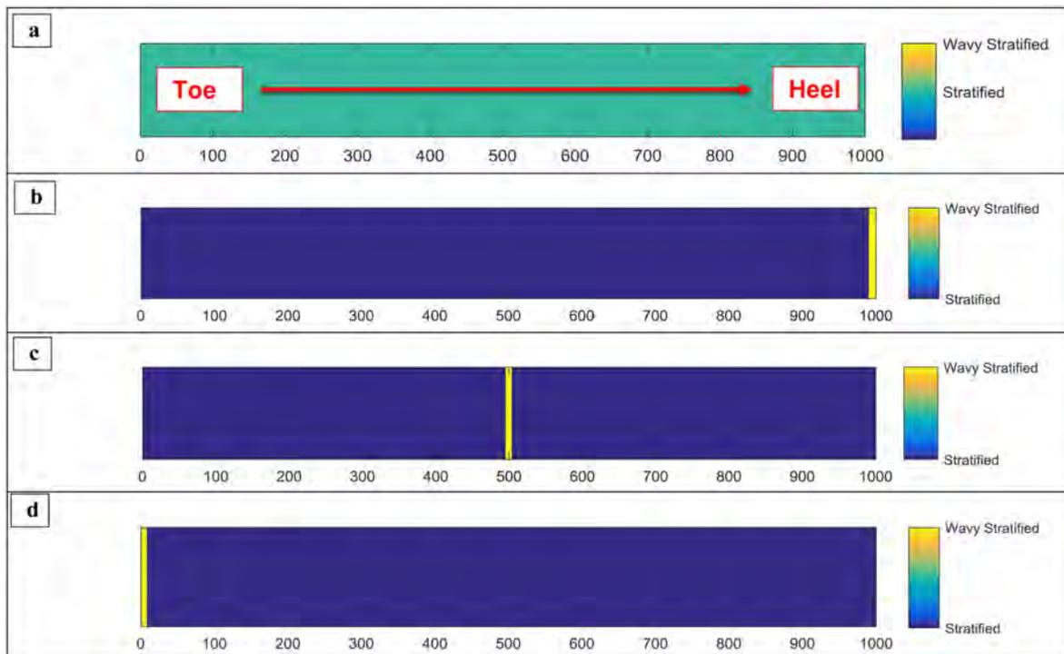
Figure 7—Flow regime along 1000 m well with standalone screen design, 7 inch diameter standalone screen; (a) no steam breakthrough, (b) steam breakthrough at heel, (c) in the middle and (d) at toe
