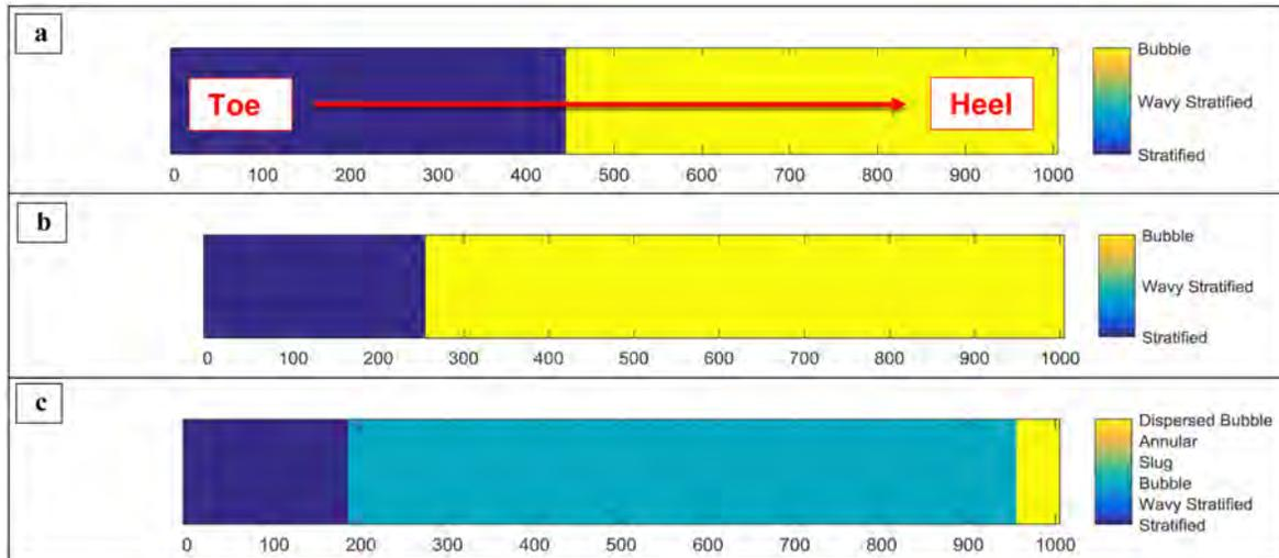
Figure 16—Flow regime along 1000 m well with liner deployed completion design, 7 inch diameter screen with no steam breakthrough; (a) liquid rate=1000 bbl/d, (b) liquid rate=3000 bbl/d, (c) liquid rate=6000 bbl/d
