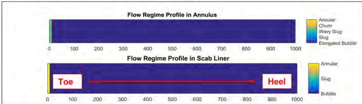
Figure 11—Flow regime along 1000 m well with scab liner design, 4 ½ inch diameter scab liner and 7 inch screen for steam breakthrough at toe; top figure is for annulus and bottom figure is for scab liner
