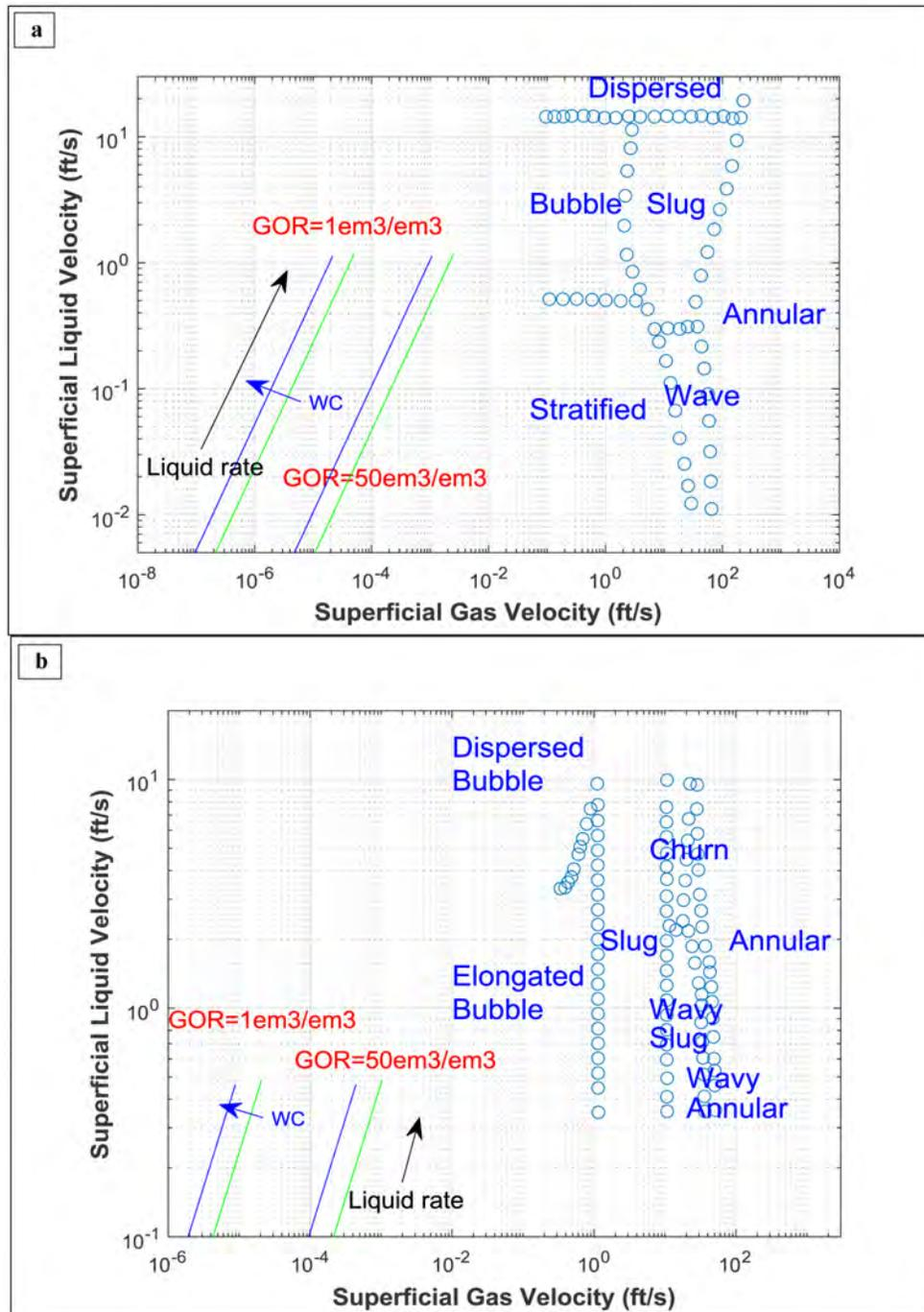
Figure 6—Flow regime charts for tubing size of 4 1/2 and annulus size of 7 inch; (a) tubing and (b) annulus
