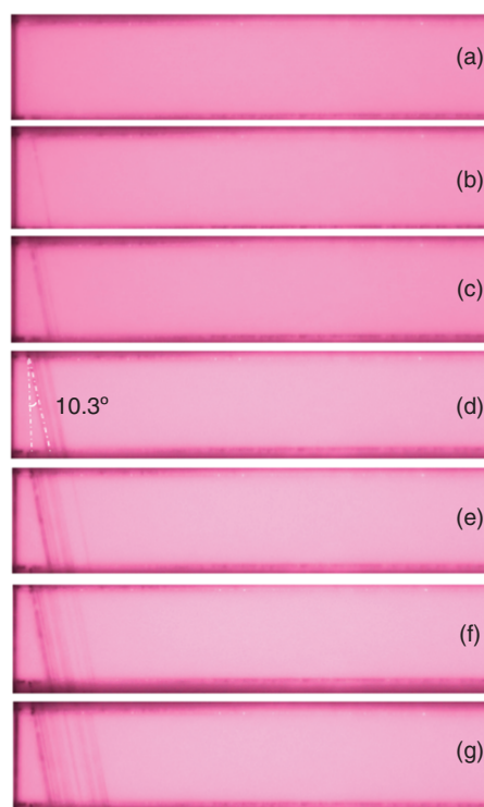
Figure 5. Sequential EL images captured from sample II near the front facet with a high magnification of 200 times at different aging times: (a) 0 h, (b) 400 h, (c) 800 h, (d) 1200 h, (e) 1600 h, (f) 2000 h, and (g) 3024 h.
