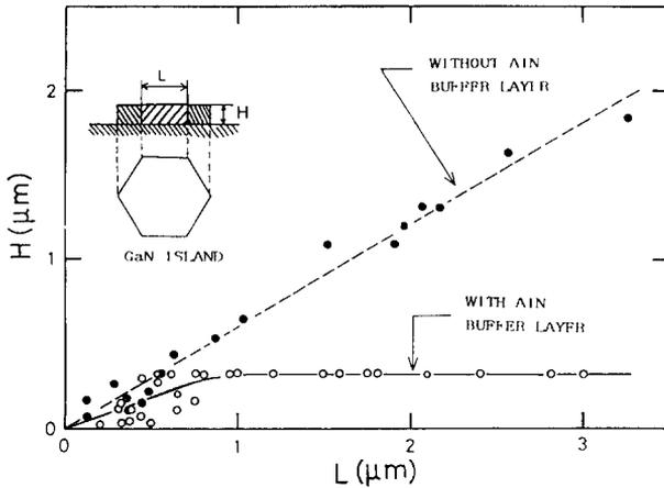
Fig 4 Horizontal vs vertical growth rates of GaN islands with and without AlN buffer layer
