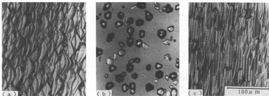
Fig 5 DIC photomicrograph of GaN grown without AlN buffer layer on sapphire substrate (a) (0001)  $3^\circ$  off-angle substrate tilted toward  $[10\bar{1}0]$ , (b) (0001) just-substrate, (c) (0001)  $3^\circ$  off-angle substrate tilted toward  $[11\bar{2}0]$
