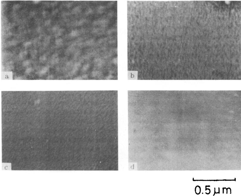
Fig 6 SEM photograph of AlN buffer layer deposited at different temperature ((a) 1100 C, (b) 1000 C, (c) 900 C, (d) 600 C)
