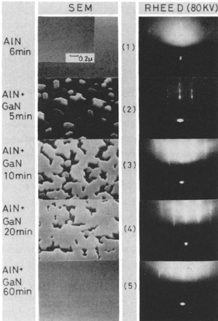
Fig 3 (a) SEM photograph and (b) corresponding RHEED pattern, of (1) AlN layer and (2–5) GaN film with different growth times
