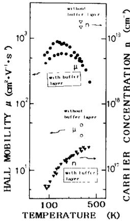
Fig 2 Electrical property of nondoped GaN films with and without AlN buffer layer
