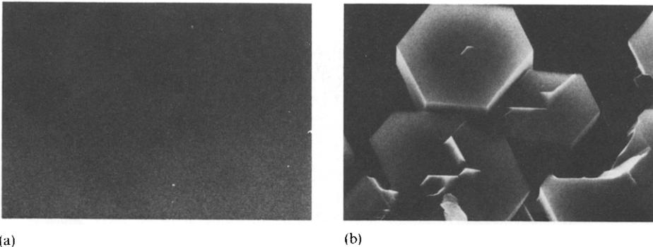
Fig. 1 SEM photograph of GaN films grown on sapphire (001) just-substrate (a) with and (b) without AlN buffer layer
