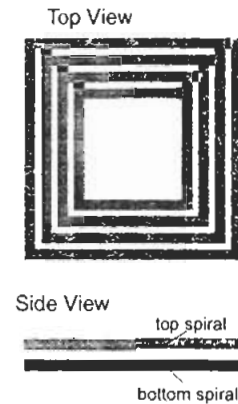
FIGURE 4.32. Stacked transformer with completely overlapping spirals.
