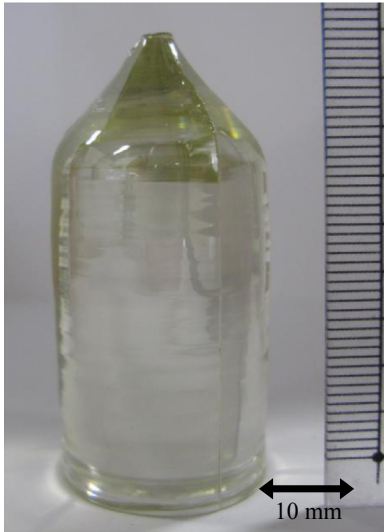
FIGURE 4.14 A cs-MgO:LN single bulk crystal grown along the Z-axis by the Czochralski method [58].
