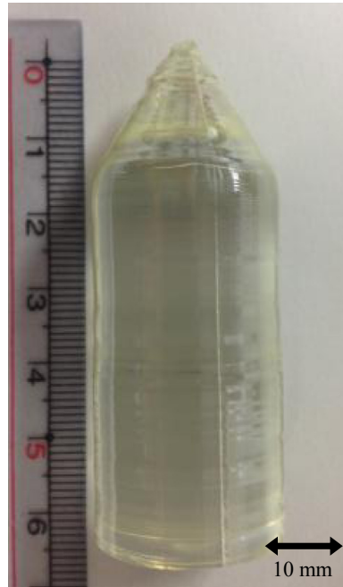
FIGURE 4.18 A cs-MgO:LT single bulk crystal grown along the Z-axis by the Czochralski method [56].
