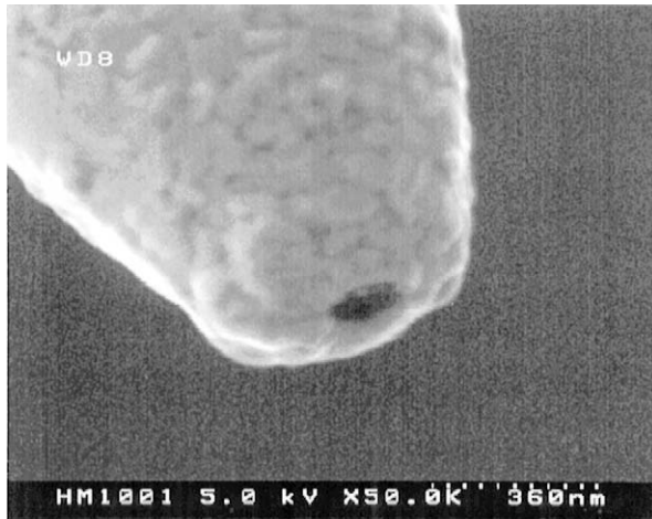
FIG. 7. Scanning electron microscope image of a metal-coated laser pulled near-field aperture probe with a tip diameter of 160 nm.
