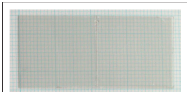
Figure 5. A 40 × 20 mm 2 homoepitaxial diamond sample produced by overgrowth of eight tiled clones. Reprinted with permission from Reference 44. © 2013 Elsevier.
