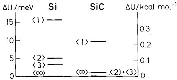
Fig. 2. Computed relative energies \Delta U for some polytype structures of Si and SiC. The structures (2) and (3) for SiC have equal energy within the accuracy of the calculations. Left scale: meV per SiC or Si 2 pair of atoms. Right scale: kcal/mol for SiC or double-mol for Si. (1 eV = 23 kcal/mol.) Results for SiC and Si from the J_n in Ref. 3.
