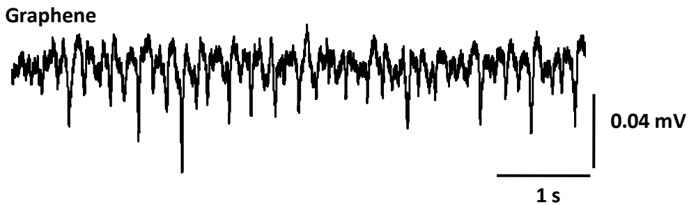
Supplementary Figure 4: Cortical EEG recorded by graphene electrode in vivo in cat model.
