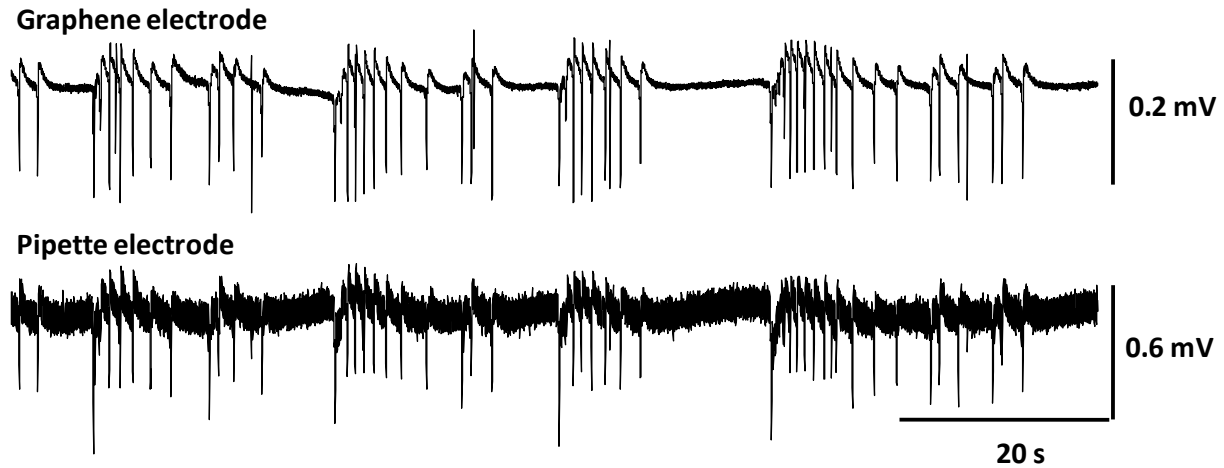
Supplementary Figure 9: Top trace shows the recordings by graphene electrode and the bottom trace shows recordings by a standard patch pipette placed close to the edge of the graphene electrode. Ictal-like activity recorded simultaneously by the graphene electrode and the patch electrode was found to be consistent.
