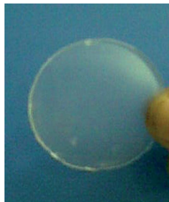
Fig. 23 Image of a \text{NaTi}/\text{EMITf}/\text{PVdF-HFP} gel polymer electrolyte film (from ref. 71). Reprinted from: D. Kumar and S. A. Hashmi, Ionic liquid based sodium ion conducting gel polymer electrolytes, Solid State Ionics , 181 , 416–423, Copyright 2010, with permission from Elsevier.
