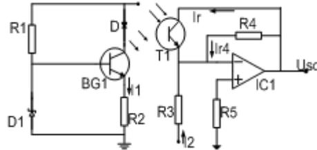
Fig.4 Coupling and amplification circuit
