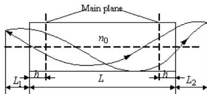
(a) Imaging of column self-focus lens
