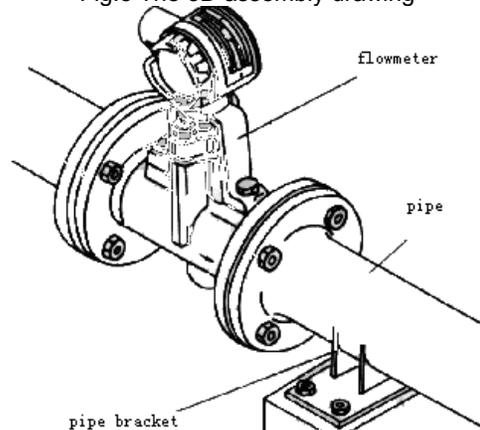
Fig.9The assembly diagram with the pipe
