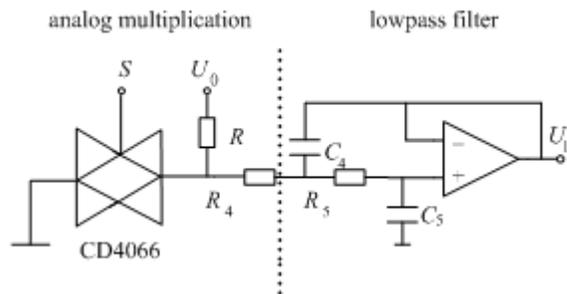
Fig.5 PSD schematic circuit
