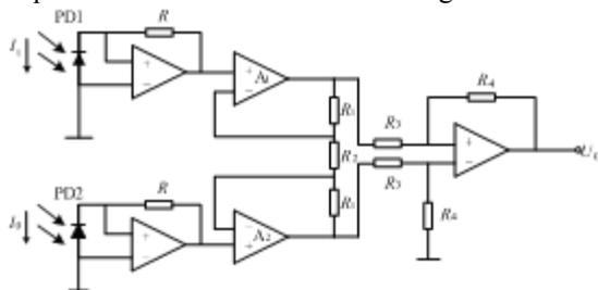
Fig.6 Differential compensation circuit for zero and temperature excursion
