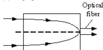
(b) Coupling of  $L = T/4$  self-focus lens and optical fiber
