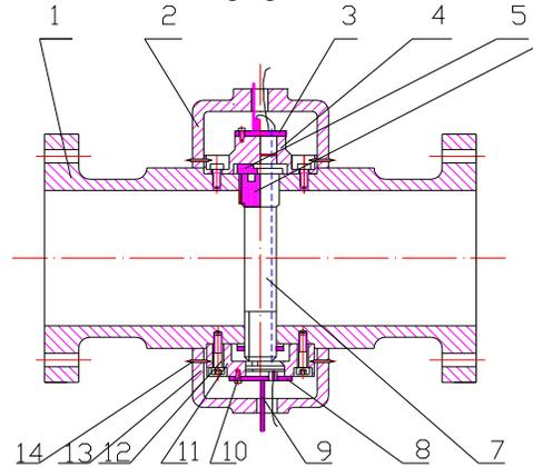
1shell 2top cover 3top baffle 4top nog 5baffle 6locating key 7vortex shedder 8bottom baffle 9optic-electro receiver 10bolt 11bottom cover 12big bolt 13bottom nog 14nut
