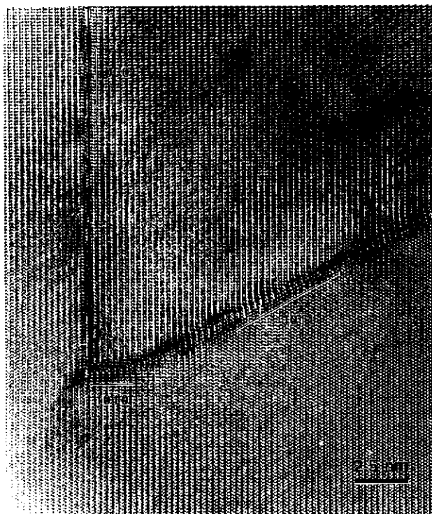
FIG. 10. A short \{10\bar{1}0\} prism facet was observed at all the intersections between curved/faceted IDB's and planar IDB's. The Burgers vector for the dislocation at the intersection is determined by the sum of the respective displacement vectors. Because the curved IDB is of variable magnitude, the Burgers vector of the dislocation would also vary. Therefore, the presence of the \approx 2.5 nm long facet would allow the Burgers vector for the dislocation to be fixed because the translation across the prism facet would be of a fixed displacement.
