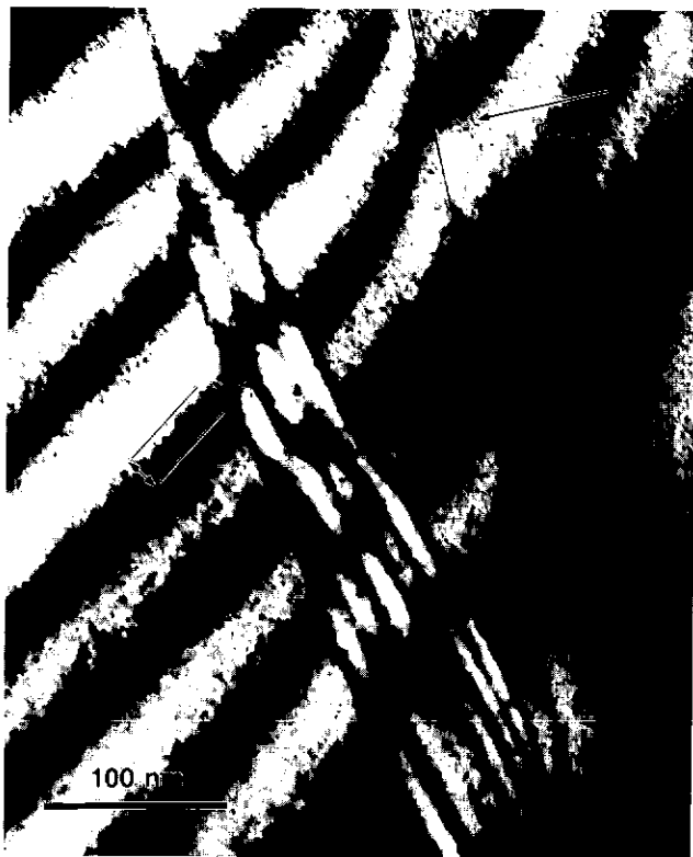
FIG. 2. A weak-beam image of a curved IDB using a g(0002) reflection. The shift in the interface fringe contrast where the extinction contours intersect the fault plane can be clearly seen with the displacement indicated by the arrow.
