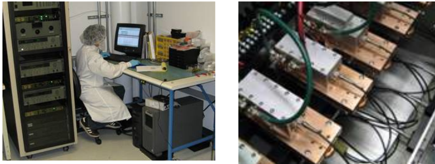
Figure 1. Overview of life-tester and details of module-level test fixturing
