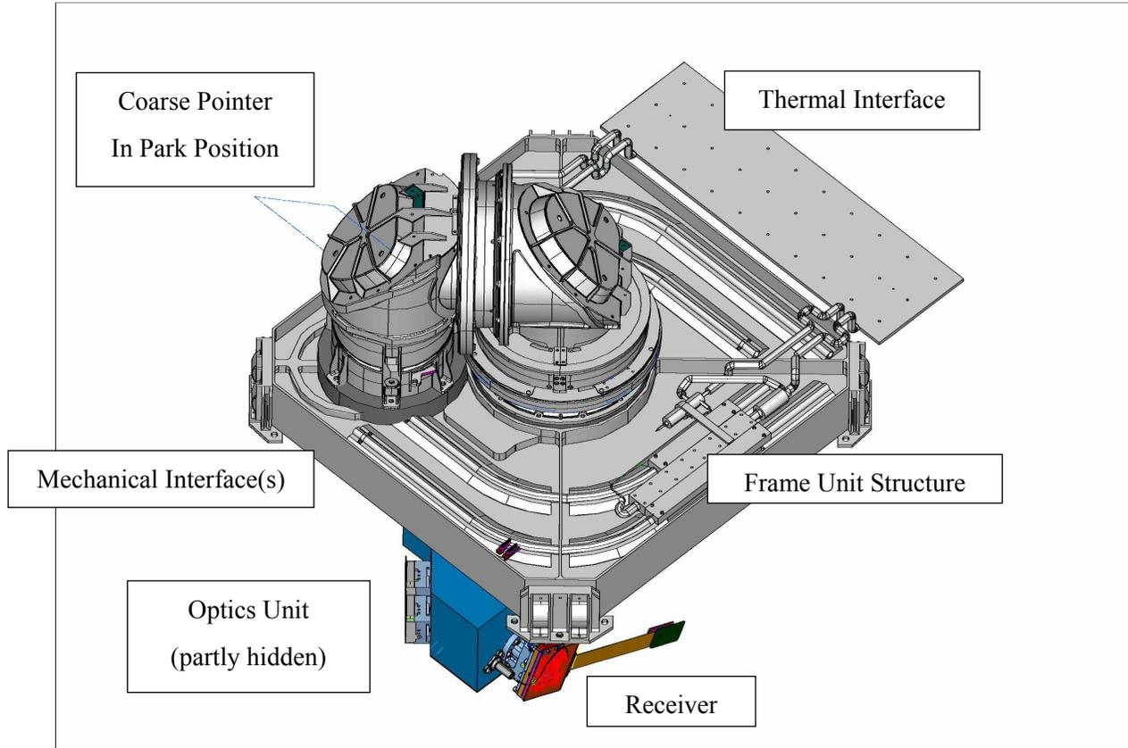
*Fig. 1: Drawing of laser communication terminal*
