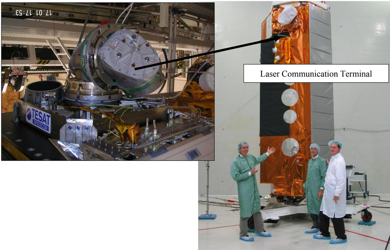
*Fig. 2: Tesat's laser communication terminal mounted on TerraSAR-X for the TerraSAR-X-NFIRE in-orbit verification*
