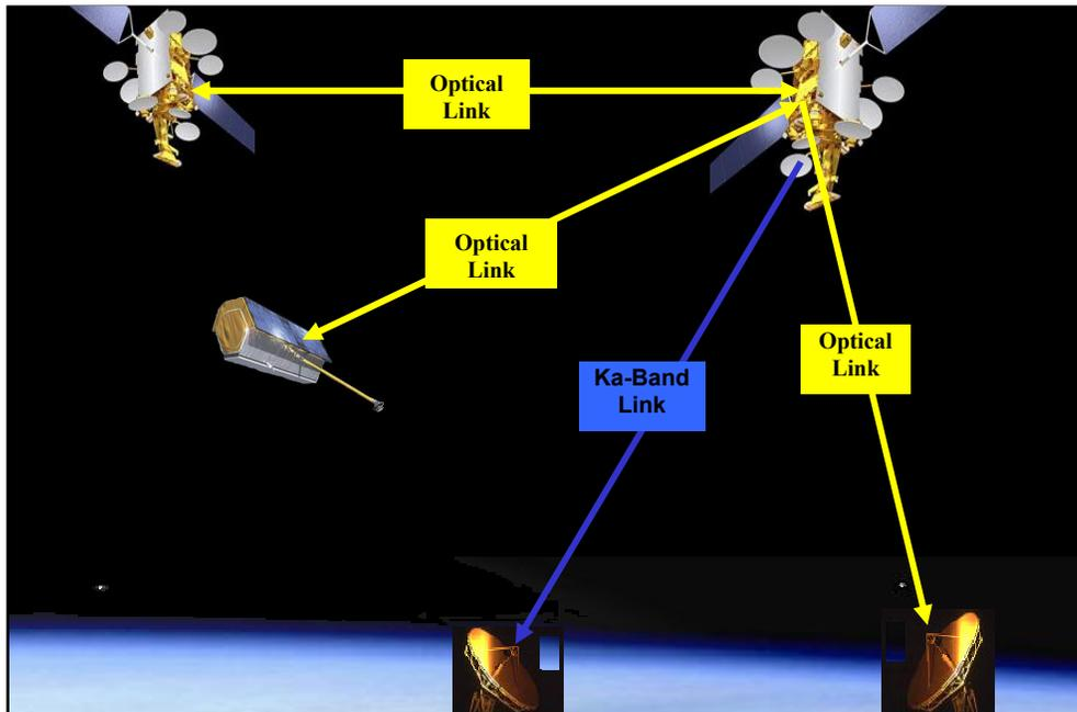
*Fig. 5: Optical data relay with Tesat's LCTs to be delivered autumn 2008 for accommodation on the LEO satellite TanDEM-X*
