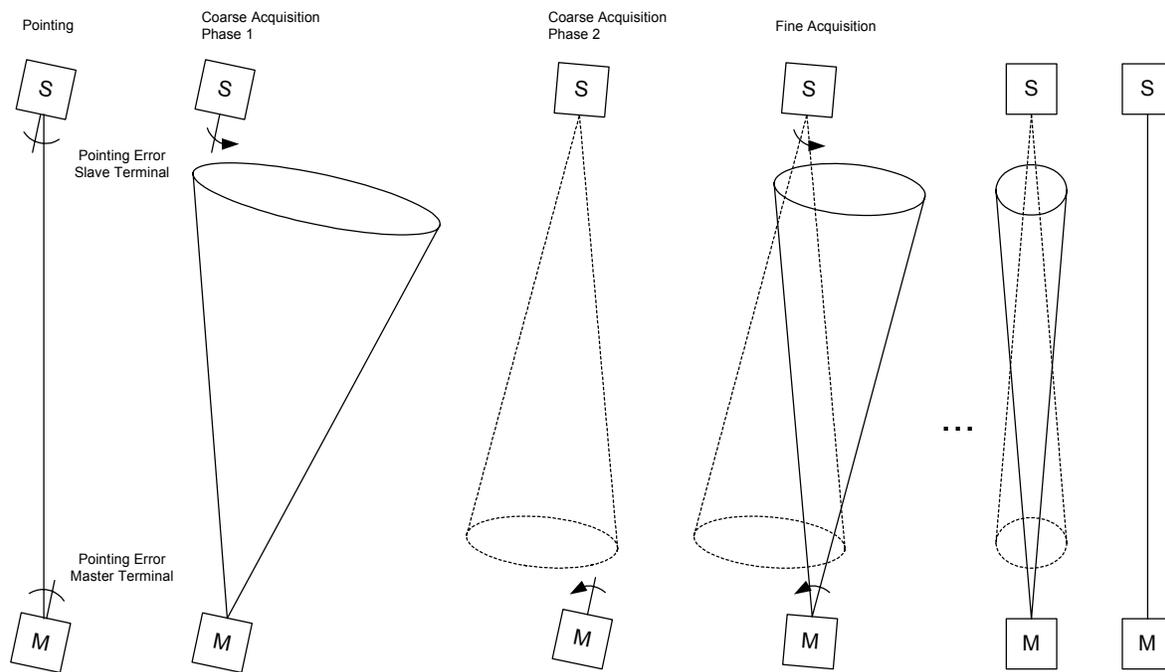
*Fig. 3: Modes of beacon-less acquisition according to a master-slave approach*
