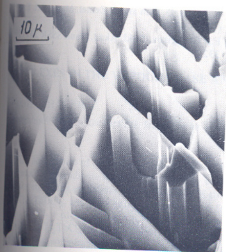
Fig. 13. Oriented growth of CdSe platelets on the (0001)CdSe substrate.
