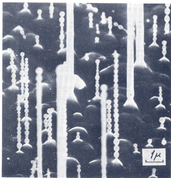
Fig. 5. Periodic instability in Si whisker growth.
