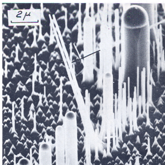
Fig. 8. Relative growth rates for GaAs whiskers of different orientations.
