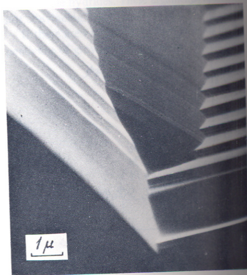
Fig. 10. Growth mechanism for the side faces of the whiskers.
