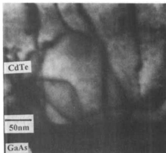
Fig. 2. TEM cross-section micrograph of a CdTe layer grown on a (211)*A* GaAs substrate
