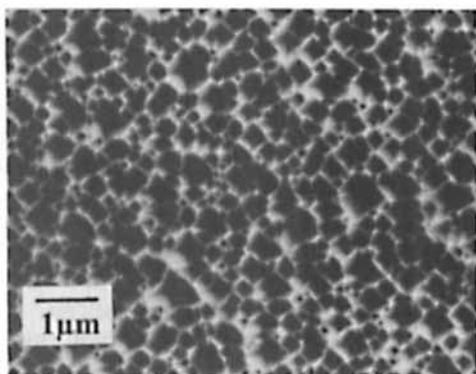
Fig. 1. Surface morphology of CdTe layers grown on (211)*A* GaAs substrates
