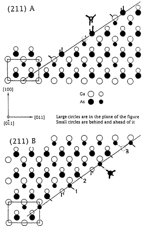
Fig. 7. Atomic structure of ideal (a) (211)*A* and (b) (211)*B* GaAs surfaces
