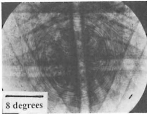
Fig. 5. Electron-channelling pattern of a CdTe layer grown on a (211)*B* GaAs substrate
