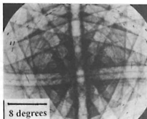
Fig. 3. Electron-channelling pattern of a CdTe layer grown on a (211)*A* GaAs substrate
