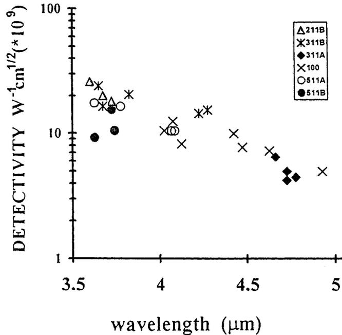
Fig. 8. Detectivity at 300 K and 10 kHz of photoconductors fabricated on MCT layers grown on GaAs substrates of various orientations and polarities
