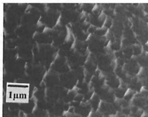
Fig. 4. Surface morphology of CdTe layers grown on (211)*B* substrates
