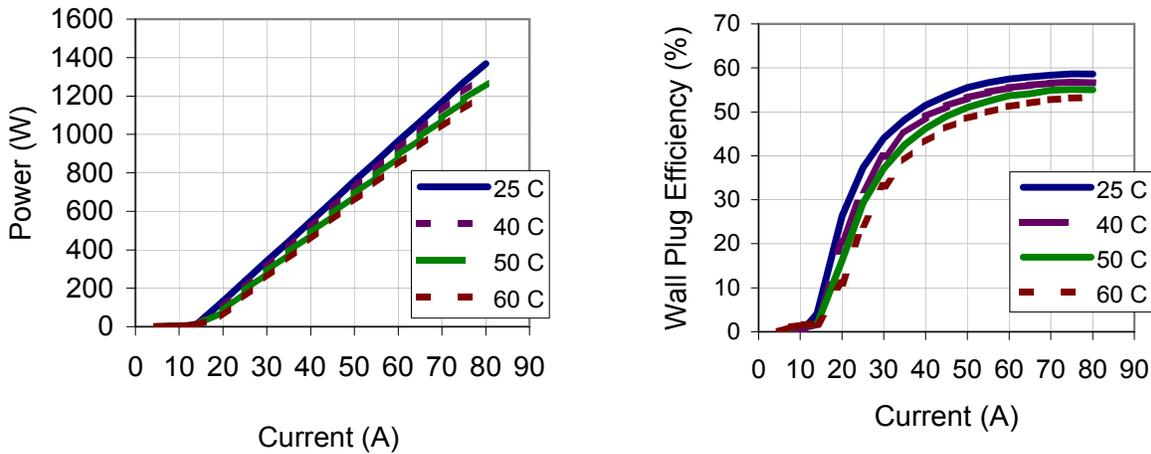
**Figure 2: Conductive-cooled 16 bar “G-stack” tested with 250 μsec pulses @ 0.5% duty cycle**
