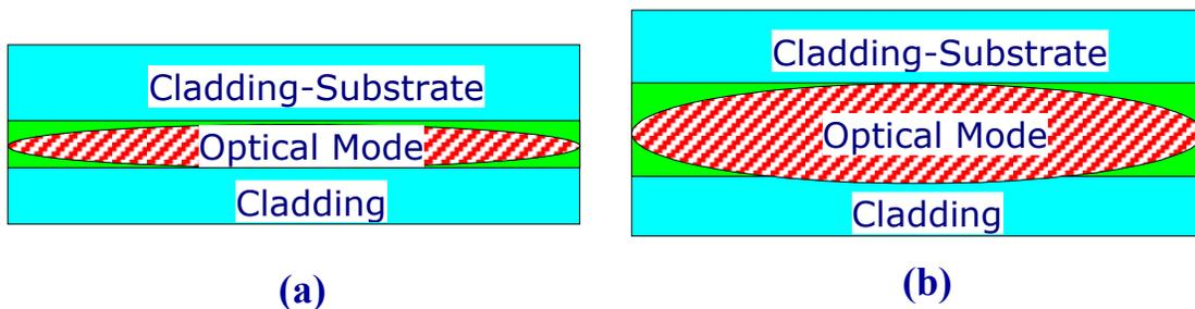
**Figure 3: (a) Traditional waveguide designed to support a single transverse mode (b) “Extended Power” design increases the waveguide thickness and expands the optical mode**
