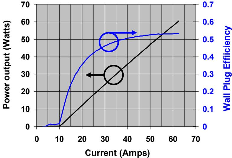
Figure 6: EP design 30% FF 1.5 mm cavity bar on CCP at 25° C
