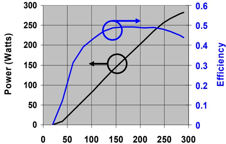
Figure 10: EP design 90% FF 1.5 mm cavity length bar tested on CCP with 500us pulses @ 50Hz at 25° C.
