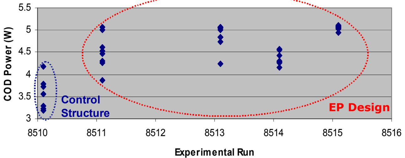
**Figure 4: Measured COD power limits of 60 μm wide 1.5 mm long single emitter devices of traditional and EP epi designs**
