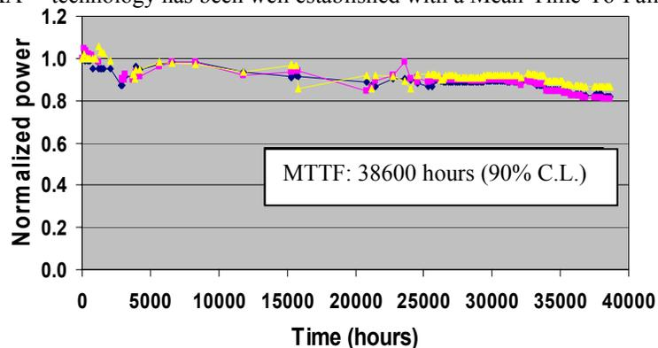
**Figure 1: 90% FF 0.6 mm cavity on conductively cooled package tested with 200  $\mu$ sec pulses @ 25% duty cycle at 80 Amps Constant Current (80 W) at 25° C.**
