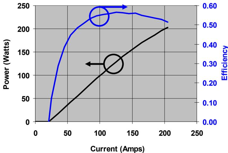
Figure 7: EP design 75% FF 1.0 mm cavity length tested CW on MCCP at 20° C
