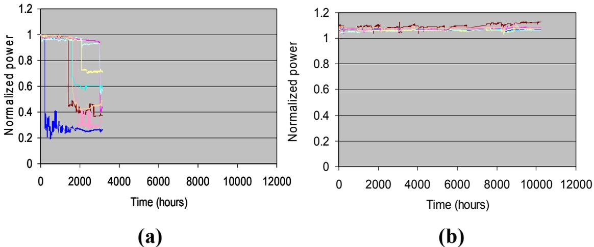
**Figure 5: (a) Life test of traditional epi design single emitters (b) Life test of EP design single emitters**
