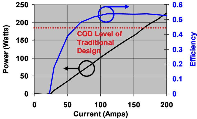
Figure 8: EP design 90% FF 1.0 mm cavity length tested on CCP, 200us pulse @ 100Hz at 20° C
