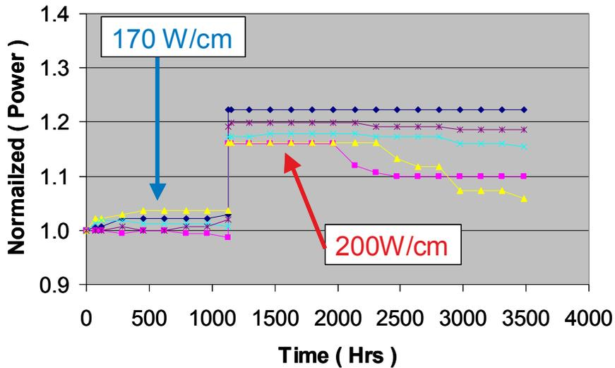
Figure 9: “Half bar” 90% FF 1.0 mm cavity length devices on CCP, 500us pulse @ 400Hz at 25° C
