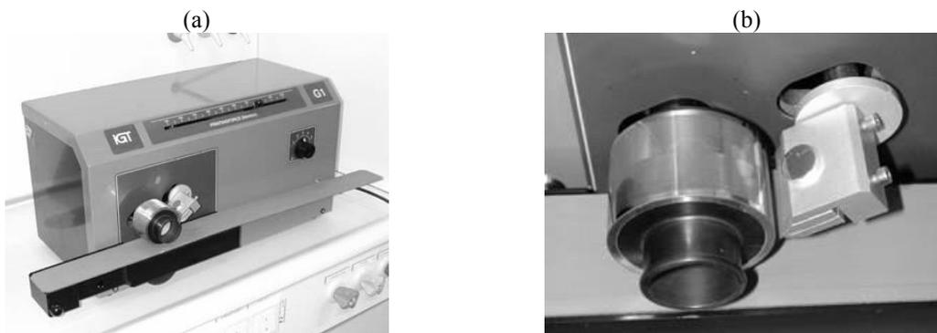
Figure 1. Photographs of (a) a table-top size gravure printer, and (b) a doctor blade and cylinder with engraved cells.
