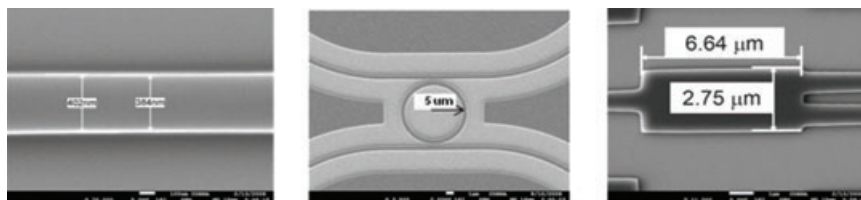
Figure 7 Passive IMOS-devices, from left to right: a) Photonic wire waveguide of 400 nm width b) Ring filter with 5 \mu\text{m} radius c) Ultra-small 1-by-2 MMI coupler.
