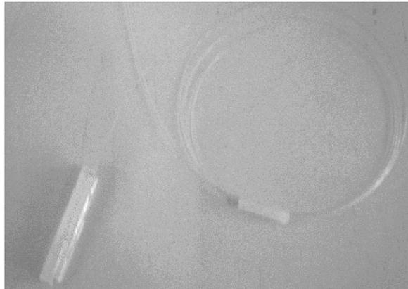
Fig. 1. FBG sensor for human respiration measurement
