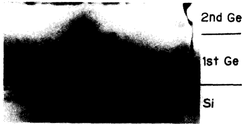
Fig. 6. A magnified cross-sectional TEM micrograph of a Ge layer (sample 8). Note that some propagating dislocations are truncated at the interface between first and second Ge layers.
