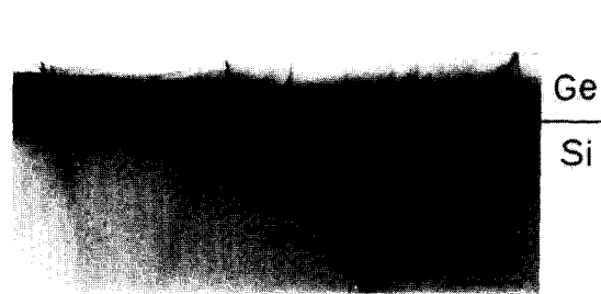
Fig. 5. A cross-sectional TEM micrograph of Ge layer (sample 8).
