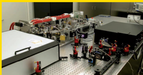
A 200 W high-power laser system developed for advanced gravitational wave detectors. The box on the left contains a 35 W front-end laser which is used to injection-lock the high-power stage (center of the photograph). The black box contains diagnostic tools to perform a comprehensive laser characterization.
