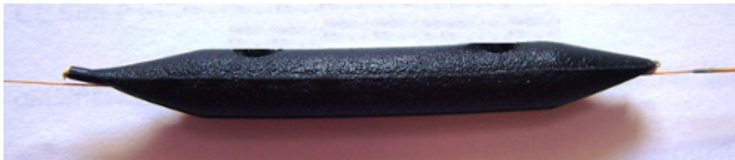
Fig. 4. Photograph of the FBG hydrophones coated with UR5041.
