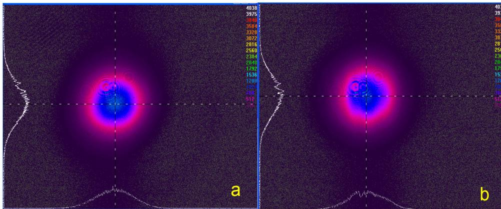
Fig.5 Far field pattern of the two free running fiber lasers (a) fiber laser1, (b) fiber laser2
