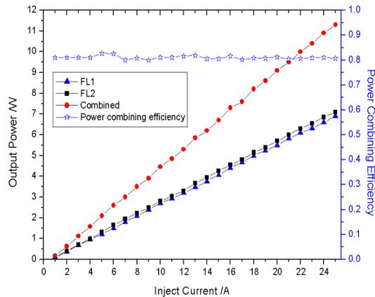
Figure 7 the change curve of the output power and the corresponding power combining efficiency before and after coherent combining of two-way fiber laser
