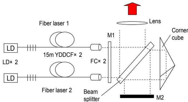
Figure 2 Mutual injection phase-locking fiber laser experimental system with an extra-cavity based on a corner-cube
