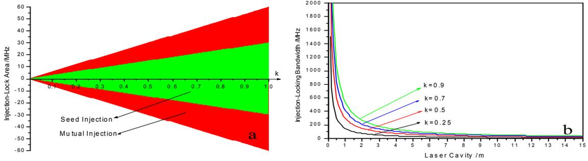
Figure 1. Comparison between single injection phase-locking and mutual injection phase-locking bandwidth(a), the rate relationship between mutual injection phase-locking bandwidth and mutual injection energy (b)
