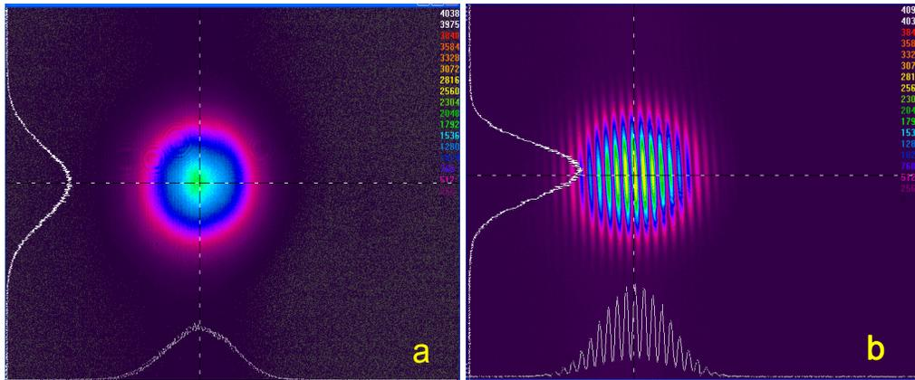
Fig.6 Far field pattern of the two fiber laser array in (a) free running, (b) mutual injection
