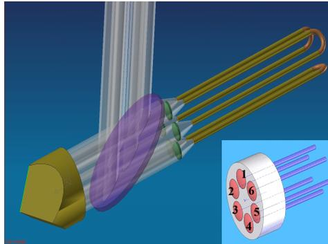
Figure 4 Program of mutual injection phase-locking fiber laser based on a corner-cube
