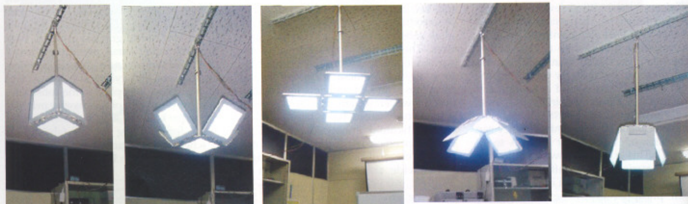
Figure 5. Recent demonstration of 140 mm × 140 mm OLED lighting panels. The panels had an operating efficiency of 5,000 cd/m 2 and a luminous efficiency of 20 lm/W.
