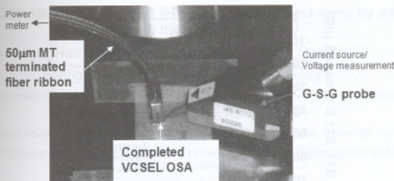
Fig. 3. Photograph of VCSEL OSA optical coupling loss measurement setup.
