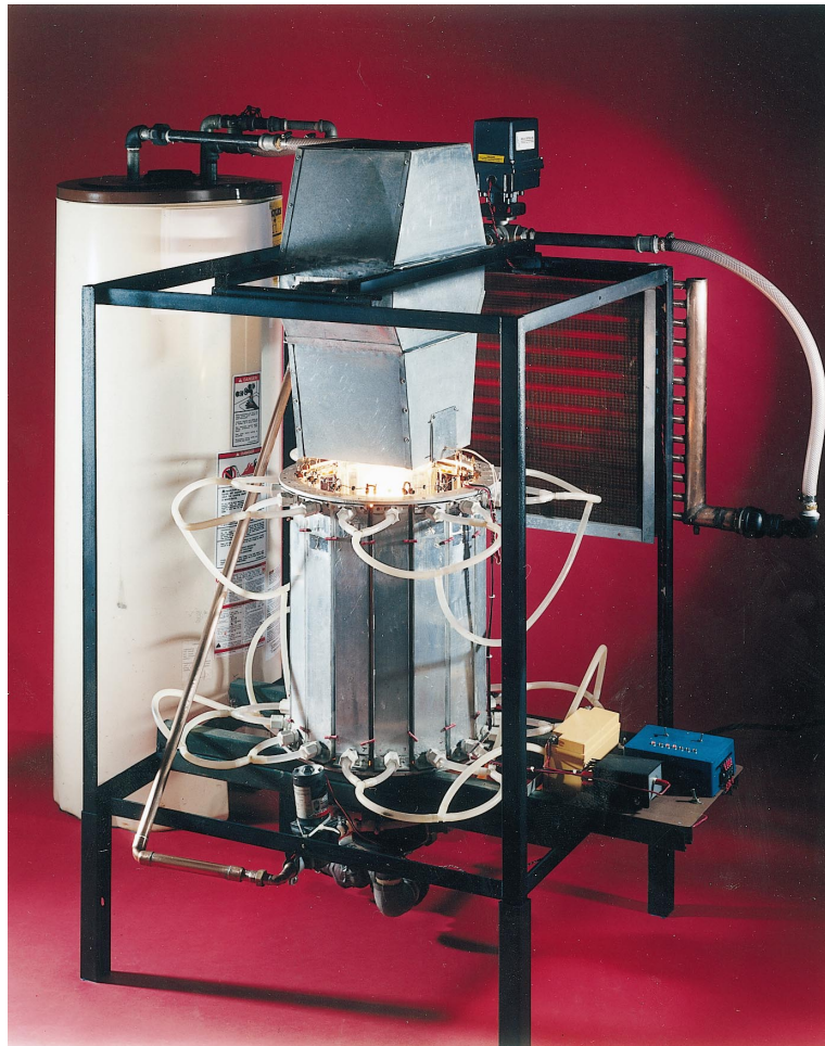
Fig. 65. Photograph of the Quantum Group, Inc., TPV hydronic/electronic TPV generator developed by Kushch et al. Reproduced by permission of the American Institute of Physics, and the author(s) [108].
