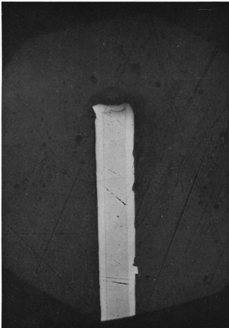
FIG. 6. Cross-sectional view of a wafer of GaAs on which Ge has been deposited. The thickness of the deposit is about 0.03 cm.
