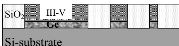
Figure 12. Schematic drawing of the epitaxial III/V layers grown on Ge virtual substrates. The thickness of the Ge layers is limited to 75 nm to enable SEG of the III/V within the STI trenches.
