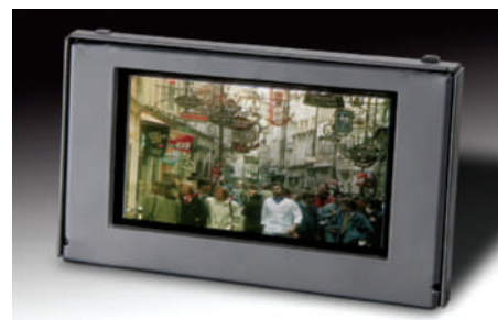
Figure 3 | This 3-inch diagonal P-OLED display has a resolution of 302,400 pixels at a pixel density of 160 pixels per inch. It was made using inks from Sumation and high-resolution ink-jet printing.
