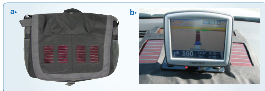
Figure 1 | Prototypes developed at Solarmer energy, where polymer solar cells are integrated with consumer products. a , A messenger bag. b , A GPS charging pad. The cells will generate power under light, extending the battery life of portable electronic devices and allow users longer periods between charging.
