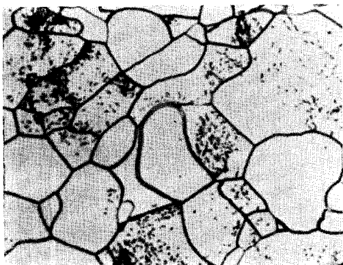
FIG. 7. Microstructure of crystal No. 5 after a 1 min anneal at 980°C and a carbon addition treatment at 770°C. \times 500 .
