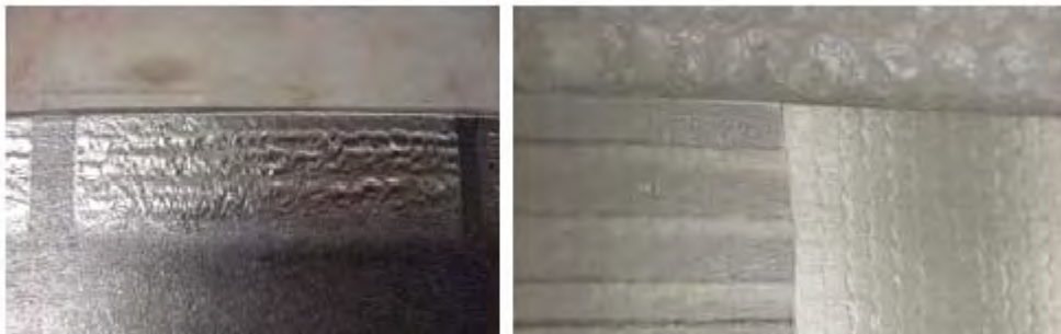
Figure 3a: 1080 steel glazed with high-power diode laser, b: 1080 steel laser peened (right side) and glazed and peened (left side)
